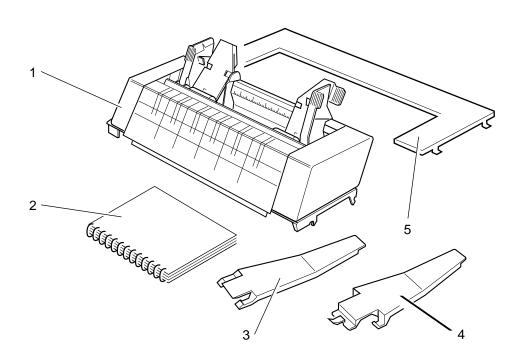
$\label{eq:2.1} {\bf 2} \quad {\rm Attach \ the \ front \ and \ rear \ stacker \ supports \ to \ the \ sheet \ feeder.}$
